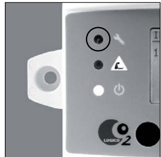
System fault indicator
