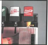
Read the ratio cup levels. Tap the ratio cup three times to release air bubbles in syrup and CO2 bubbles in water. Place it on a LEVEL surface and read immediately. If the levels are equal or within one line above or below each other, the ratio is within the correct range (Go to Step #14). If the levels are out of the correct range, the ratio needs to be adjusted (Go to Next Section). RINSE and DRY the ratio cup after each test.
