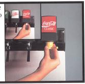
**Pill the separator.** Tap the valve lever or flow button quickly to fill the separator with syrup and water. This procedure expels trapped air in separator.
