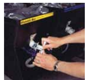
Quick disconnect bag connectors make bag changes fast and easy
